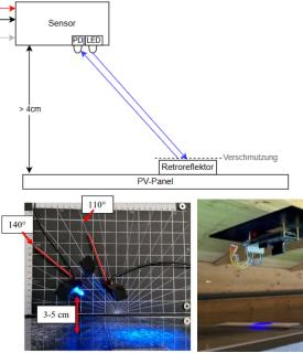
**Figure 5:** The optical reflection of a blue LED light is measured as the functional principle of the soling sensor and the indoor experimental test setup and the position within the BOX on top of the PV module is shown in the photographs below.
