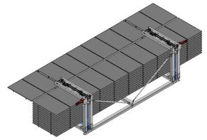
Figure 3: URBANBOX Concept of horizontal and vertical PV module movement.
